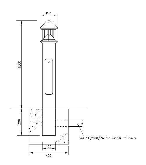
DW WINDSOR 'RIGA' BOLLARD With anodised louvre - no backshield
