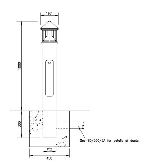
DW WINDSOR 'RIGA' BOLLARD With anodised louvre - no backshield
