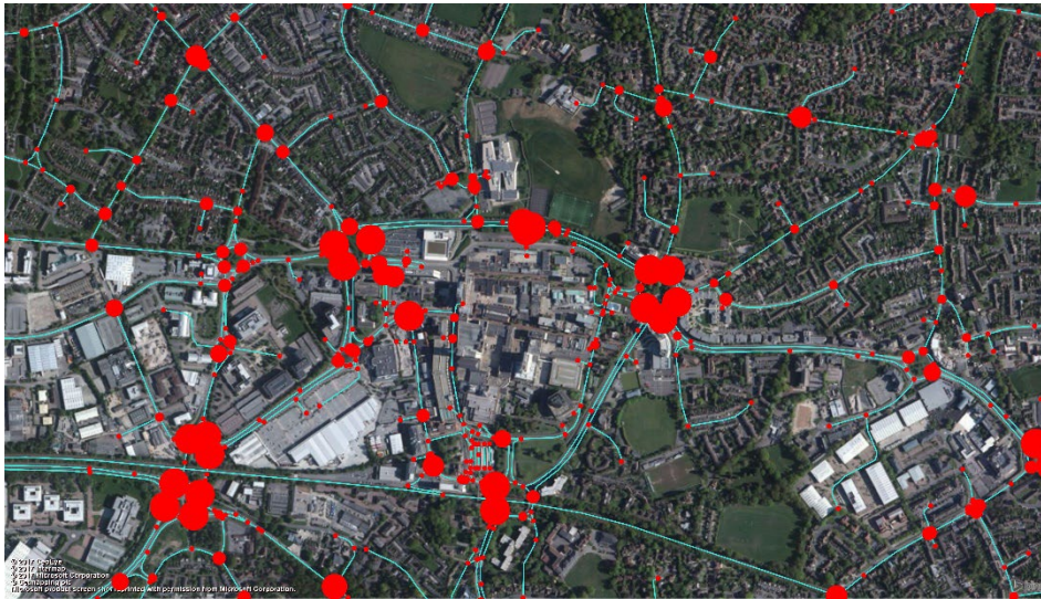
Figure 4.1. Display showing junction delay
