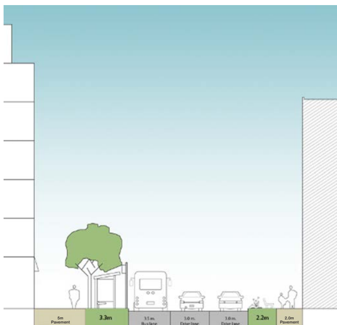
Figure 8.30: Section through Station Road
